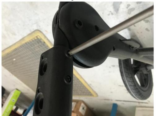
Remove Brake assembly by unscrewing the brake from the legs.
