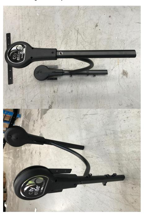
Use Bull Nose pliers to remove rivet studs. (Multigrip pliers to re-assemble)
