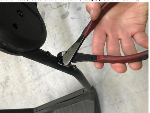
Unscrew screws from inside mounting bracket
