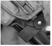
1. Line up the hood clips so that the hole (A) lines up with stud (B) on the chassis and push the clip onto the stud (B)
