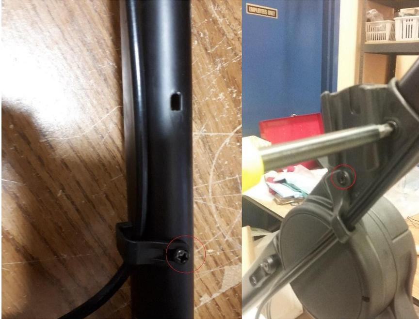
3- Remove the 2 side bolts to disassemble the bar between the 2 rear wheels
