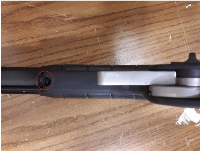
2 – Remove the brake cable guides along the upper handle.
