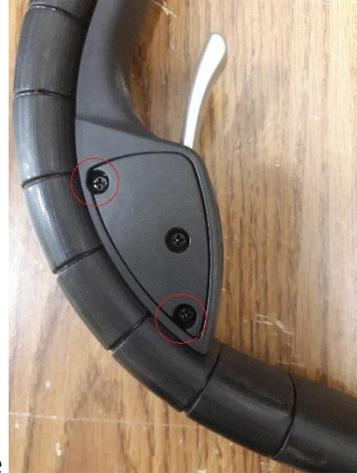
By removing the 2 screws (circled in red) on the underside
